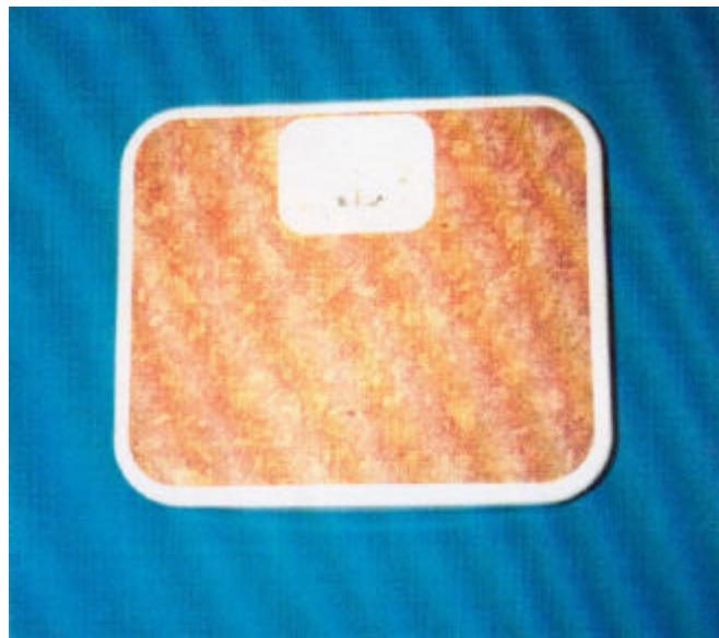
FIGURE 1: EKS, Sweden, analogue bathroom scale. Its measuring range is 0-120 kg and the dial is marked in the divisions of 0.5 kg.
