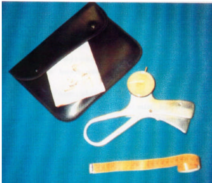
FIGURE 3: The Holtain Skinfold Caliper, Holtain Ltd., Crosswell, Crymch, Dyfed SA41 3UF UK. It has been designed to produce a constant pressure of 10 gmm -2 between its jaws over its entire operating range (0-40 mm) and the dial is marked in divisions of 0.2 mm.
