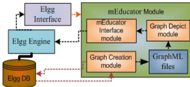
Fig. 2. Abstract architecture of the graphical representation module.
